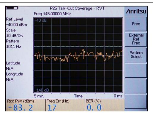
Figure 17-3. RSSI vs Time with Limit Line
