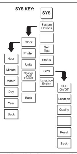
Figure 2-17. SYS Key Menu in Power Monitor (External Detector) Mode
