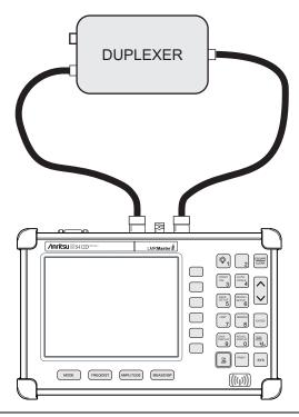
Figure 9-2. Transmission Measurement Connections
