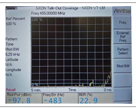
Figure 19-3. BER vs Time with Limit Line
