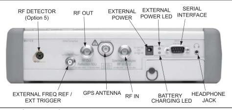
Figure 2-1. S412D Test Connector Panel
