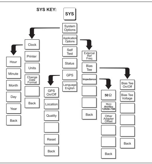
Figure 2-23. SYS Key Menu in Interference Analyzer Mode
