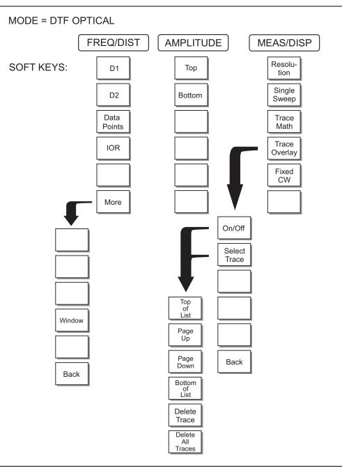
Figure 2-9. Distance to Fault Mode Optical Menu
