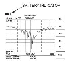
Figure 2-34. LMR Master Battery Indicator
