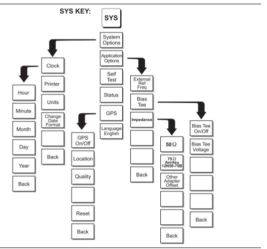
Figure 2-20. SYS Key Menu in Transmission Measurement Mode
