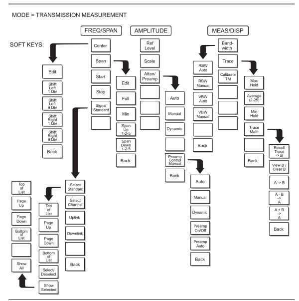
Figure 2-19. Transmission Measurement Mode Soft Keys
