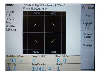
Figure 18-1. Constellation Diagram Definition and View
