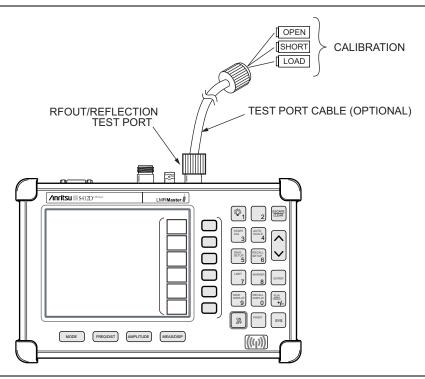
Figure 3-2. Calibration Setup
