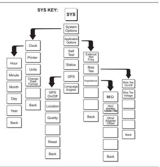
Figure 2-15. SYS Key Menu in Power Meter Mode
