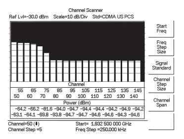
Figure 13-3. Example of Channels Displayed in Bar Graphs with Channel Step Size = 5
