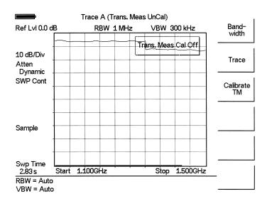
Figure 9-1. Uncalibrated Narrowband Trace
