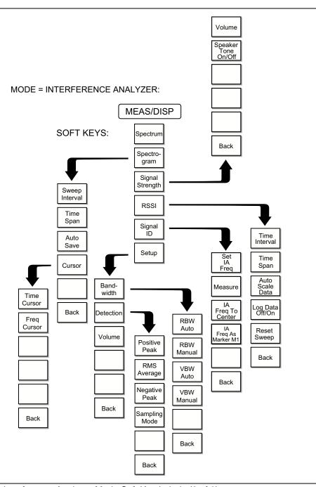
Figure 2-22. Interference Analyzer Mode Soft Key Labels (2 of 2)
