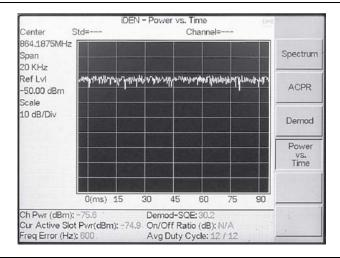
Figure 15-3. Power vs. Time Display
