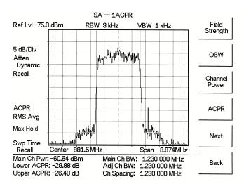
Figure 5-6. Adjacent Channel Power Measurement
