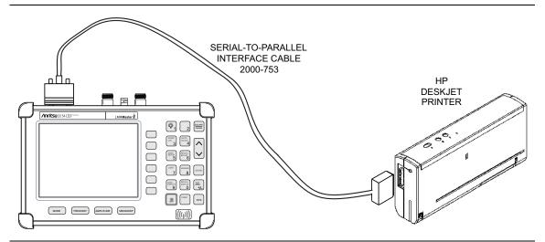
Figure 3-4. LMR Master Printer Setup
