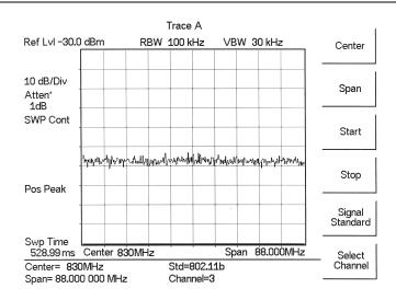
Figure 5-10. Signal Standard and Channel Selected
