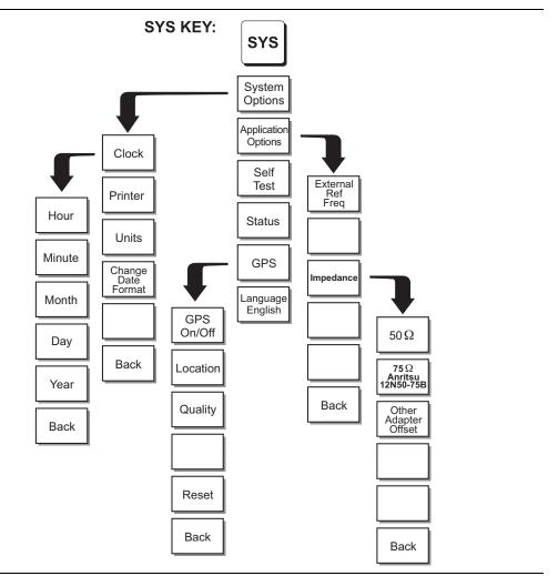
Figure 2-25. SYS Key Menu in Channel Scanner Mode
