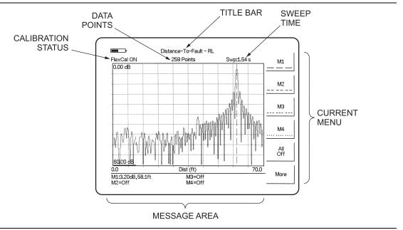
Figure 2-2. S412D Distance-To-Fault Display Overview
