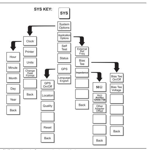
Figure 2-13. SYS Key Menu in Spectrum Analyzer Mode
