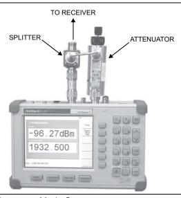
Figure 14-1. CW Signal Generator Mode Setup
