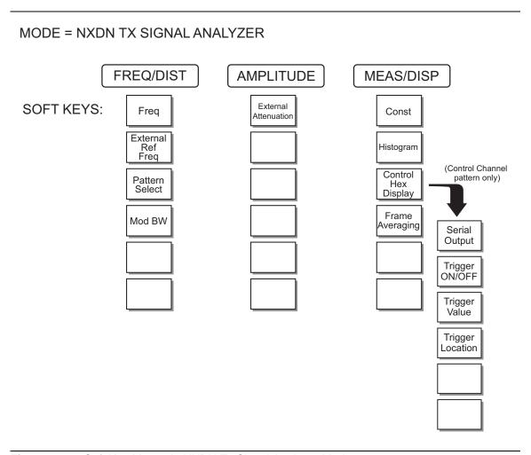
Figure 2-31. Soft Key Menus in NXDN Tx Signal Analyzer Mode
