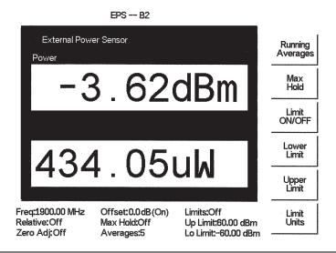
Figure 8-1. High Accuracy Power Measurement Display
