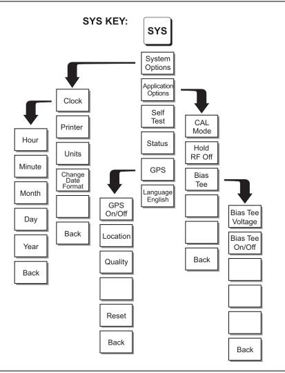
Figure 2-10. SYS Key Menu in Cable and Antenna Analyzer Mode
