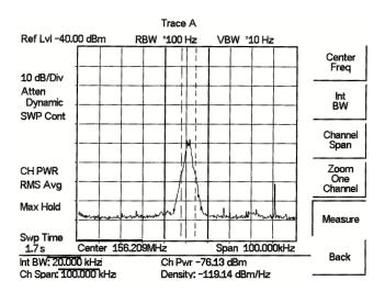
Figure 5-5. Channel Power Measurement
