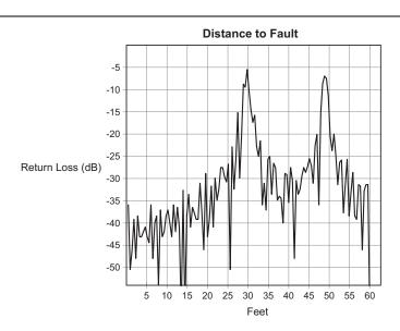
Figure B-1. Rectangular Windowing Example
