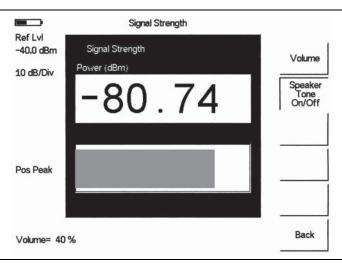
Figure 12-2. Signal Strength Display
