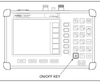
Figure 3-1. LMR Master ON/OFF Key
