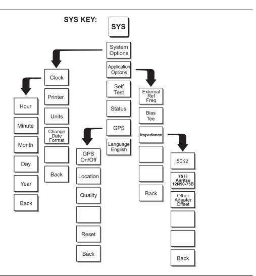
Figure 2-27. SYS Key Menu in CW Signal Generator Mode
