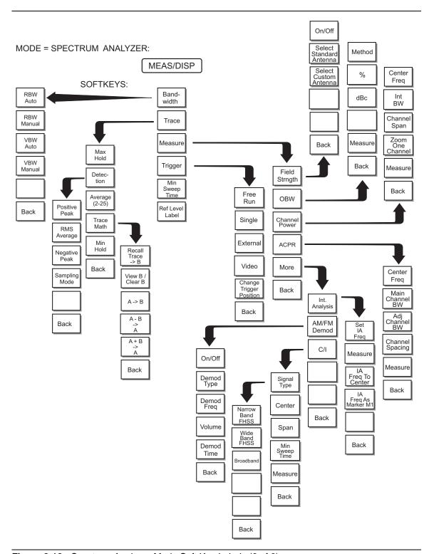
Figure 2-12. Spectrum Analyzer Mode Soft Key Labels (2 of 2)
