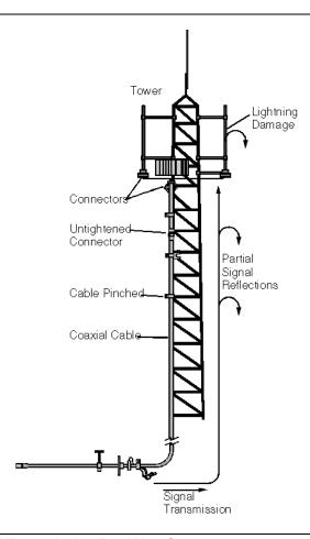
Figure 4-1. A Typical Transmission Feed Line System
