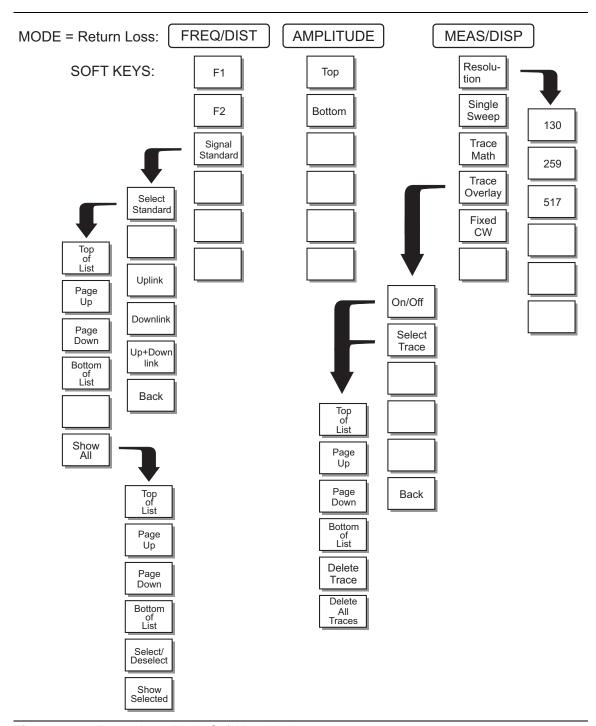
Figure 2-7. Return Loss Mode Soft Key Labels
