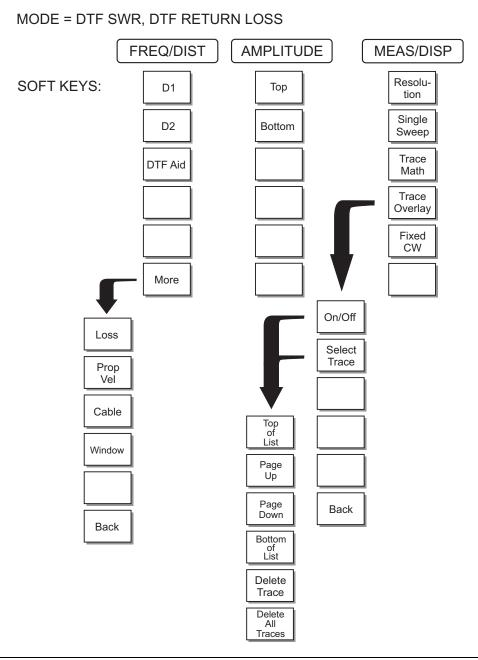
Figure 2-8. Distance to Fault Mode Soft Key Labels
