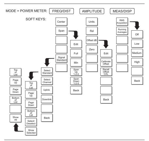
Figure 2-14. Power Meter Mode Soft Key Labels
