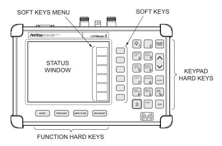
Figure 2-4. S412D LMR Master Front Panel
