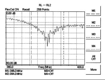
Figure 4-5. Antenna Return Loss Trace
