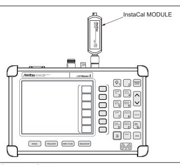
Figure 3-3. InstaCal Module Calibration
