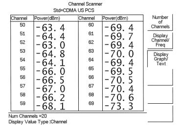
Figure 13-2. Example of Channels Displayed in Text Format
