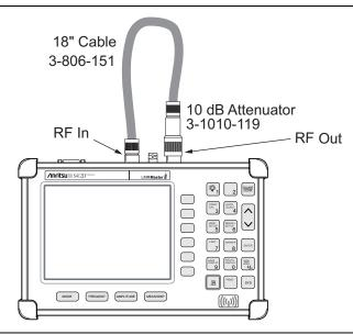
Figure 6-1. Setup for Normalizing the Trace
