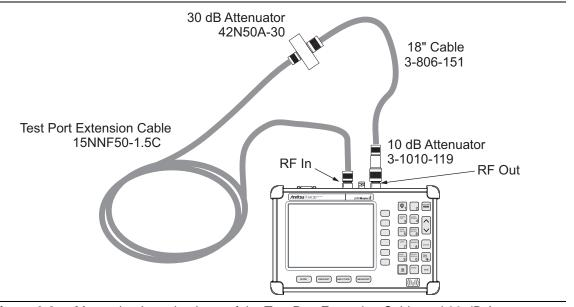
Figure 6-2. Measuring Insertion Loss of the Test Port Extension Cable and 30 dB Attenuator
