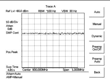
Figure 5-1. Preamplifier Off
