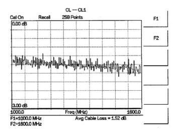
Figure 4-3. Typical Transmission Line Cable Loss Trace
