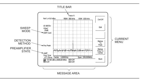
Figure 2-3. S412D Spectrum Analyzer Mode Display Overview
