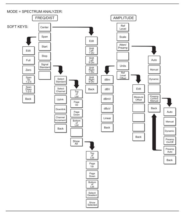
Figure 2-11. Spectrum Analyzer Mode Soft Key Labels (1 of 2)
