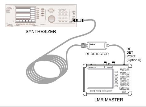
Figure 7-1. S412D LMR Master Power Monitor Setup
