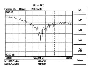
Figure 4-2. Typical System Return Loss Trace
