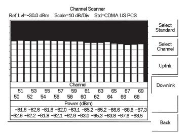
Figure 13-1. Example of Channels Displayed as Bar Graphs
