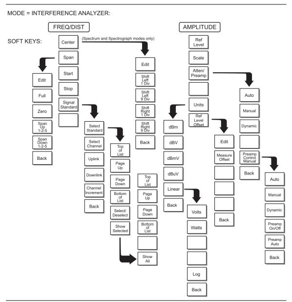
Figure 2-21. Interference Analyzer Mode Soft Key Labels (1 of 2)
