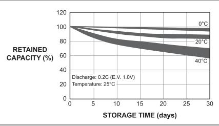
Figure 2-35. NiMH Battery Storage Characteristics
