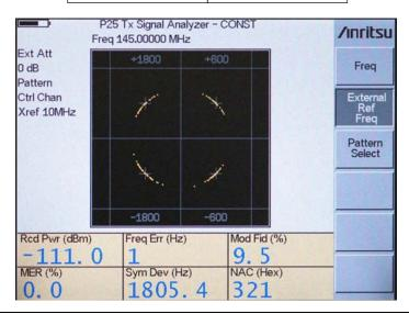
Figure 16-1. Constellation Diagram Definition and View
