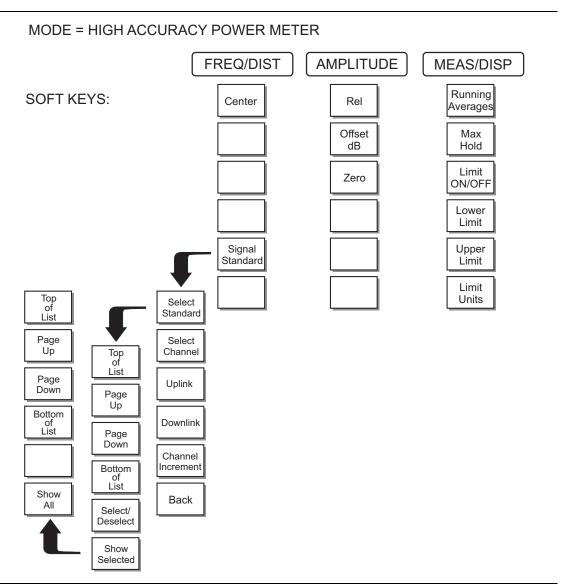
Figure 2-18. High Accuracy Power Sensor Mode (Option 19) Soft Keys
