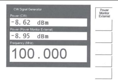
Figure 14-2. Operation with Option 5, External Power Monitor
