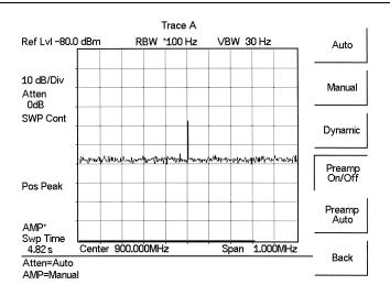
Figure 5-2. Preamplifier On
