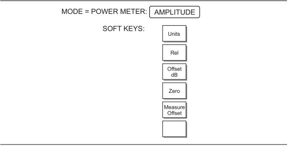
Figure 2-16. Power Monitor Mode (Option 5) Soft Keys
